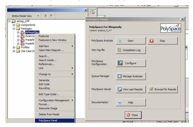
The PolySpace Panel opens. The PolySpace Panel is the interface to the PolySpace UML Link RH within Rhapsody.
